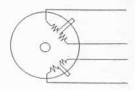
Windings in parallel for high speed/smaller torque
