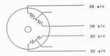
Connection of 8 wire motors Windings in series for high torque/low speed
