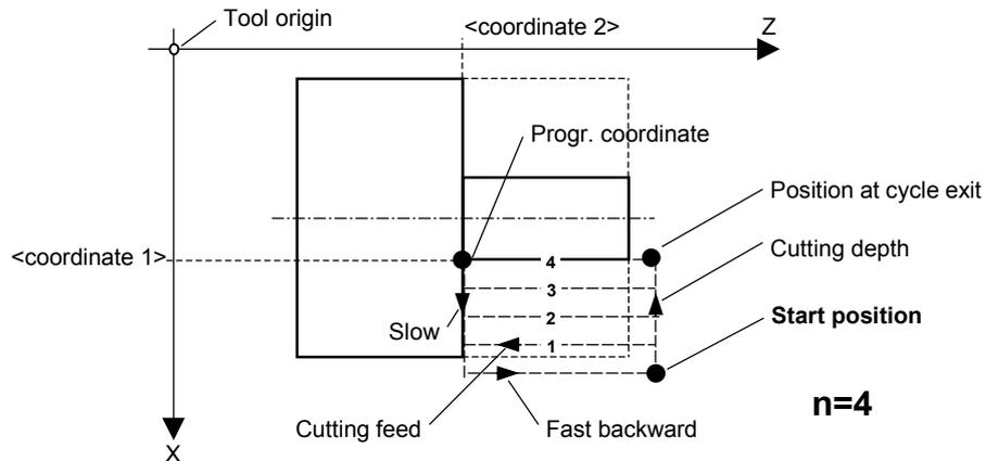
Figure 5-4 : Turning cycle CYL
