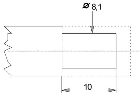
Figure 7-3 : Rough Machining
