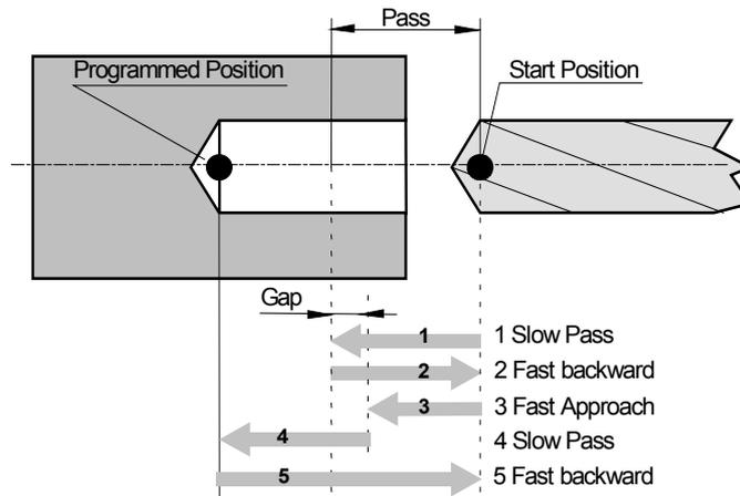
Figure 5-6 : Drilling with Peck cycles
